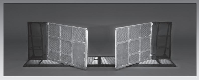
The mega exit is the largest door or gateway in the Mojo Barrier range of doors. It consists of two doors which open up to an overall width of 3.00 meters, allowing emergency vehicles or trucks to have access to or cross an installed barrier line or have quick exit possibilities. The doors swing both ways and can be opened quickly by a single manual operated lever to provide fast access.
